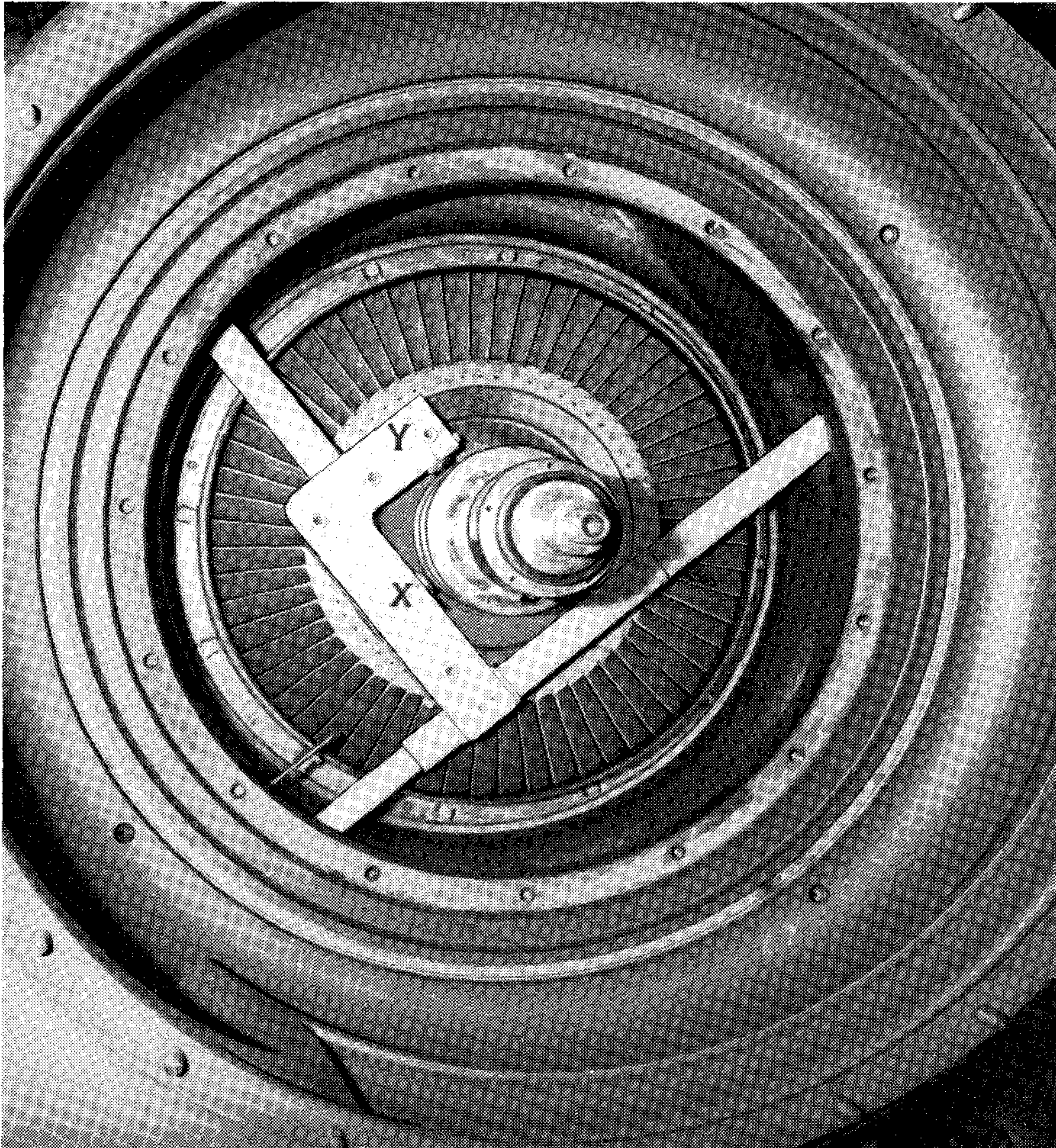
Fig.4. The supporting rig with the displacement transducers
